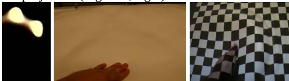
Figure 4: Left: finger tips fused together. Middle: ripples caused by a user's touch. Right: Distortion caused by rippling effect.
